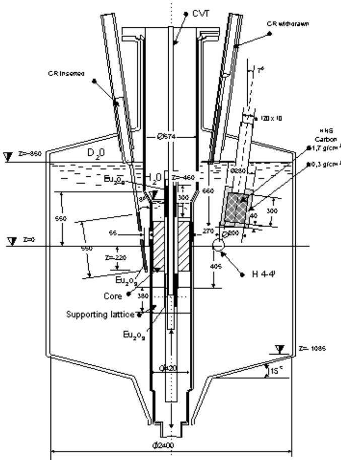
Fig. 2. Scheme of core in heavy water reflector.
