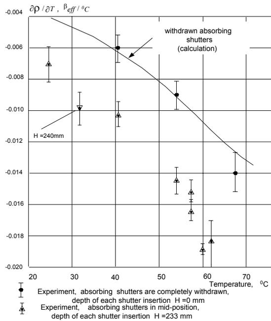
Fig.5. Temperature reactivity coefficient versus temperature
