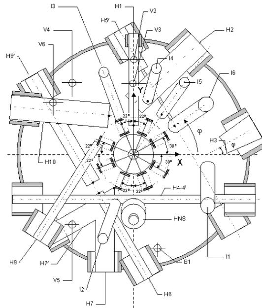
Fig. 3. Scheme of neutron beam tubes
