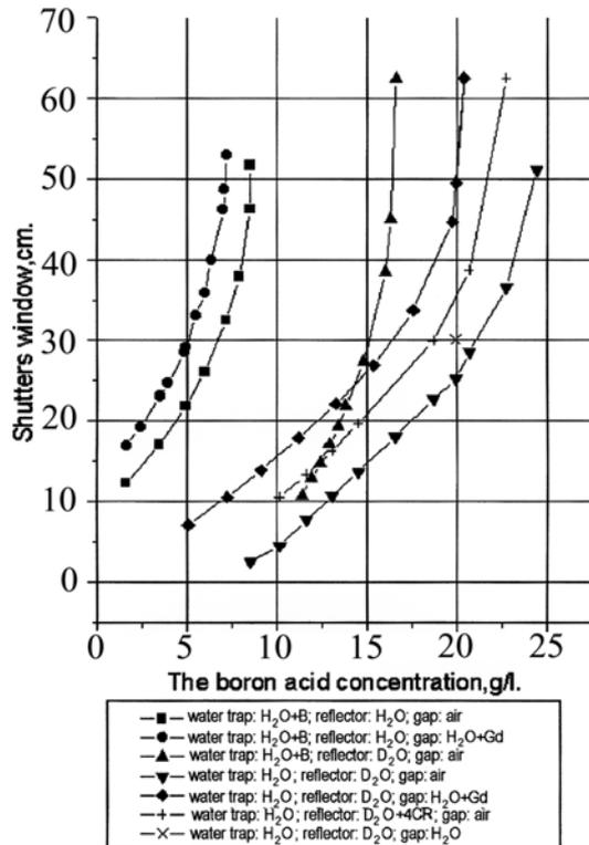
Fig. 4. Dependence of size of window between shutter absorbers on concentration of boric acid at critical state
