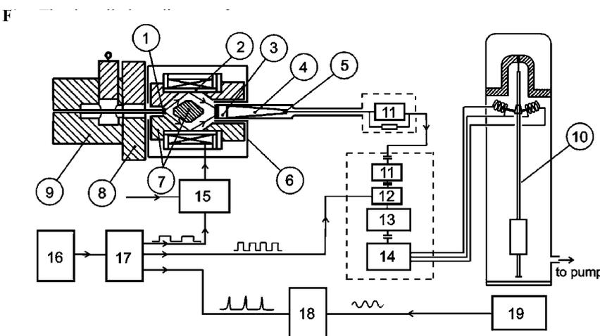
clock, 18 is phase meter, 19 is photoelectric system
