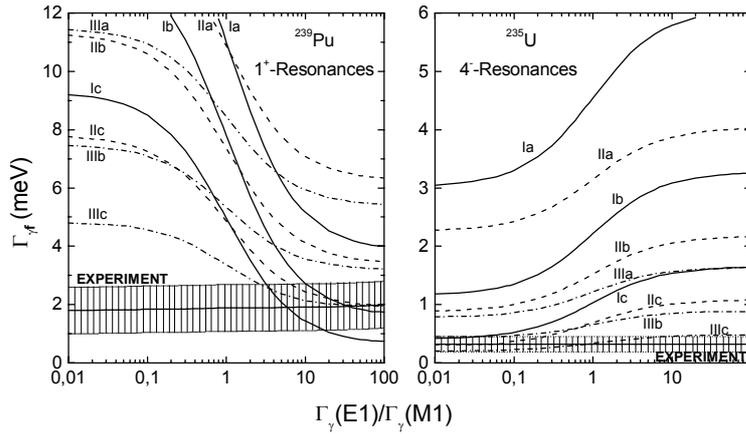
**Fig. 2.** Experimental and calculated widths  $\Gamma_{\gamma f}$  for  $1^+$ -resonances of  $^{239}\text{Pu}$  and  $4^-$ -resonances of  $^{235}\text{U}$ . Calculation model:
