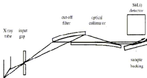
Fig. 5. Schematic view of the X-ray spectrometer with a parallel beam
